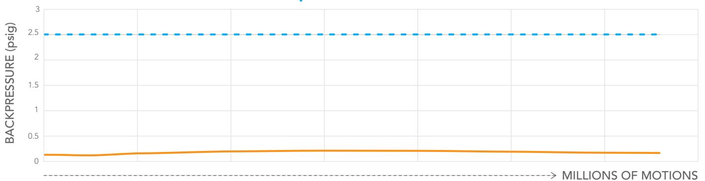
**Figure 5.** Our valve development process tests the durability of sealing surfaces for blockages that can increase system backpressure over time. From this plot of the average of 20 valves cycled with a 1X PBS solution at 80 µL/sec over millions of cycles, it is seen that there are minimal increases to the system backpressure, demonstrating material ruggedness and performance.
