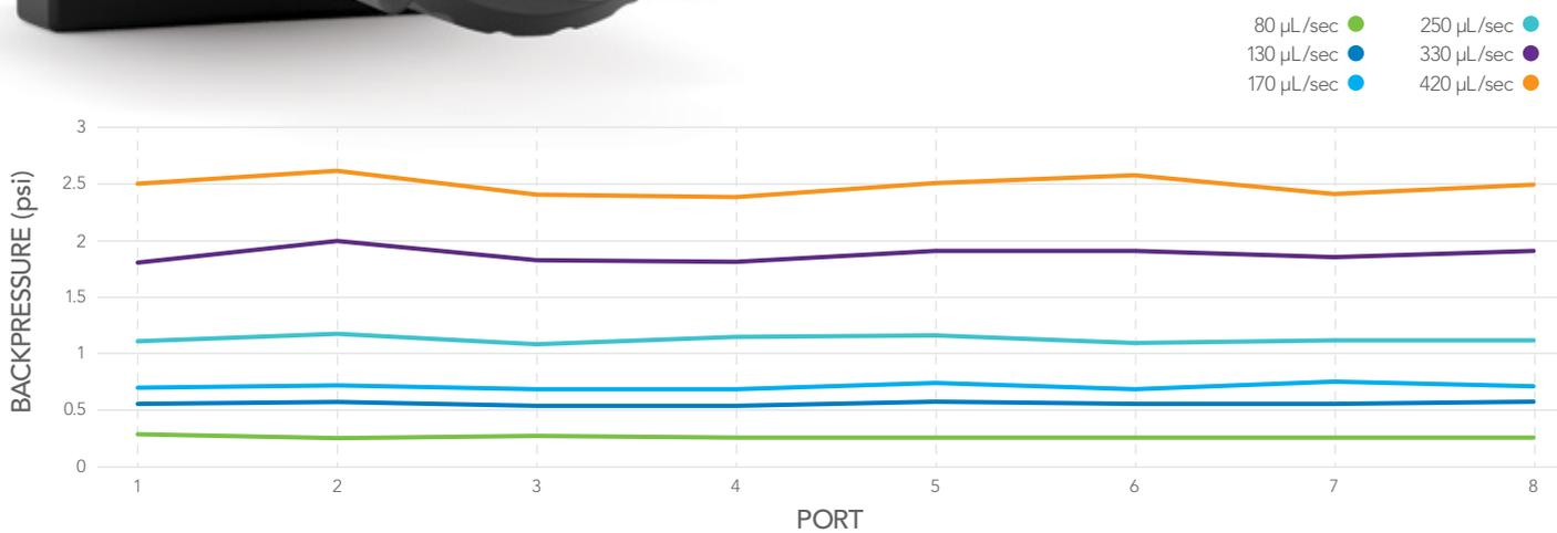
**Figure 2.** All selector valve designs are thoroughly tested to ensure best in class port-to-port reproducibility. As demonstrated, regardless of the flow rate selected (80 µL – 420 µL/sec, 20 – 22°C, 1X PBS), all ports on the TitanHP 8/9 valve offer consistent, reliable fluidic distribution, giving you confidence even in your most challenging applications.
