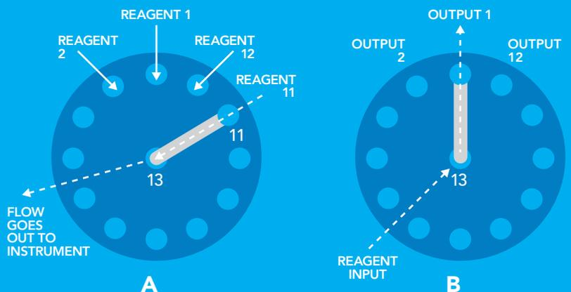
**Figure 1.** Selection valves offer the discrete connection of multiple fluids to a common center output (A) or can be used to direct fluids to different flow paths in the instrument (B). All valves are customizable to your specific fluid distribution needs, whether integrated on a push or pull flow system. Customization information can be found on page 8.
