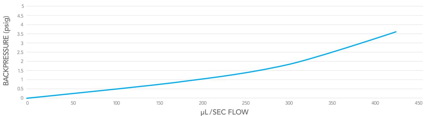
**Figure 3.** Understanding the relationship of valve backpressure to flow ensures you meet the pressure requirements for your system design. This chart represents the relationship of flow and backpressure, tested at 20 – 22°C with a 1X PBS solution. Should you have requirements that necessitate lower backpressure at higher flows, contact us for a custom valve solution.
