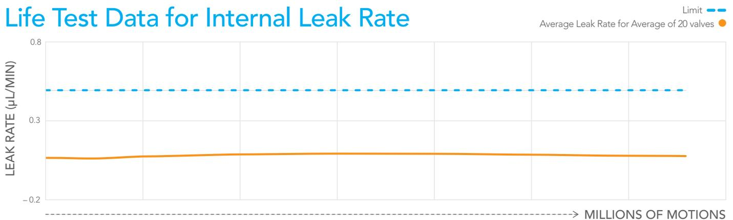
**Figure 4.** During development valve sealing materials are tested to ensure long lifetime and robust performance. This graph illustrates the average of 20 valves cycled with a 1X PBS solution over millions of cycles. Interval testing looks for internal port-to-port leakage. The rugged sealing surfaces did not suffer from scoring or internal leak failures over the course of the run.
